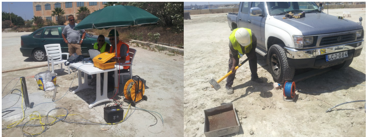
Figure 19 - Execution of the downhole seismic test in Borehole 20
