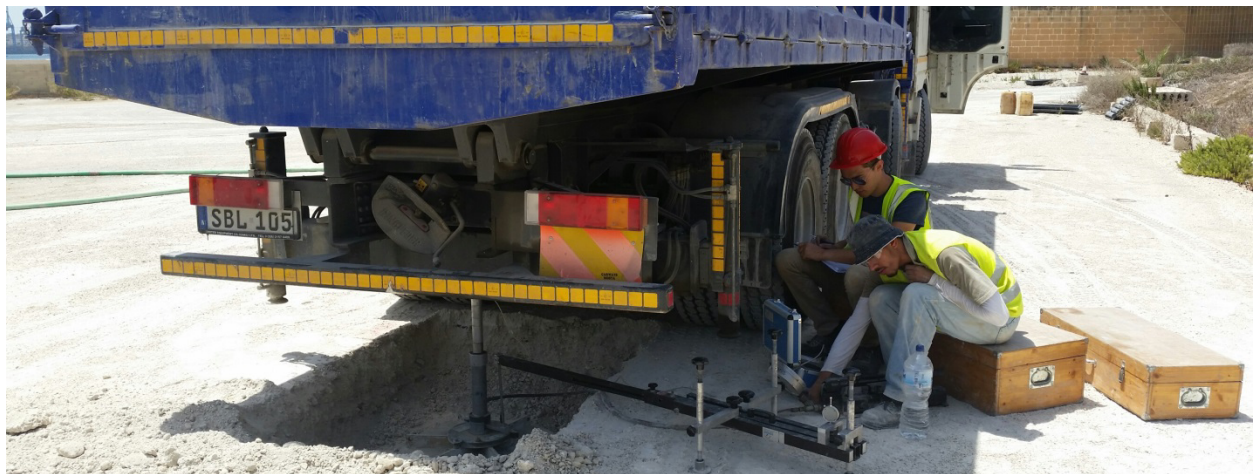
Figure 28 - Plate loading test using the large 762mm dia. plate at location 3.
