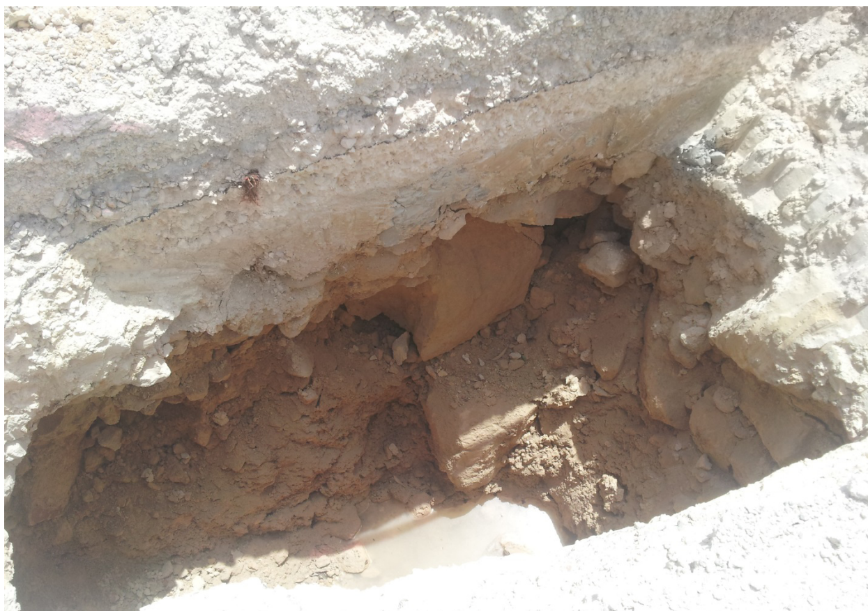
Figure 32 - Rock fill in trial pit 1 – note well-compacted upper layers and thin horizon of bitumen binder.
