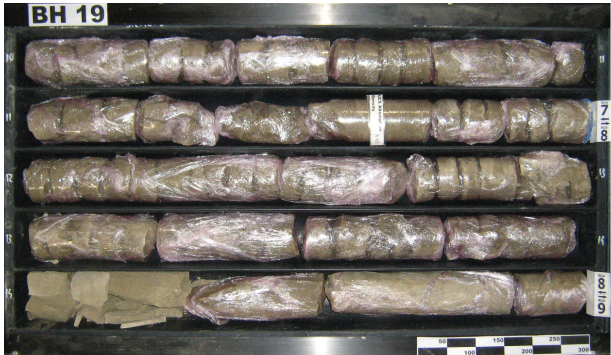
Figure 35 - example of transversally fractured sections of borehole core from the marl layer
