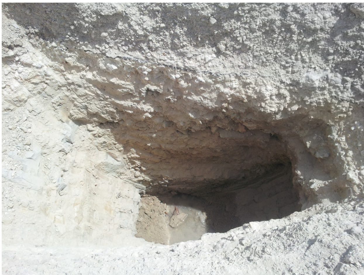
Figure 31 - Upper layers of sandy gravel (with thin layers of bituminous binder) and underlying compacted marl rock fill
