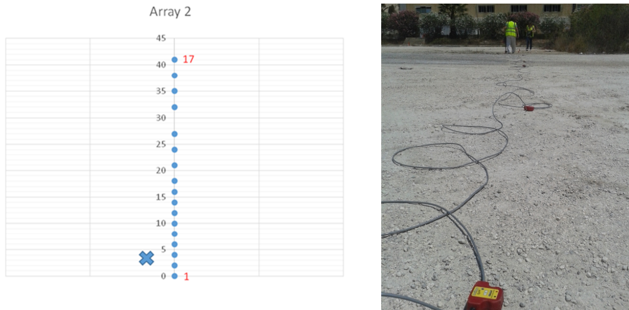
Figure 22 - Configuration and setup of array 2. Again, the numbers in red show the geophone numbers while the 'X' marks the place where the 3-component measurements were taken.
