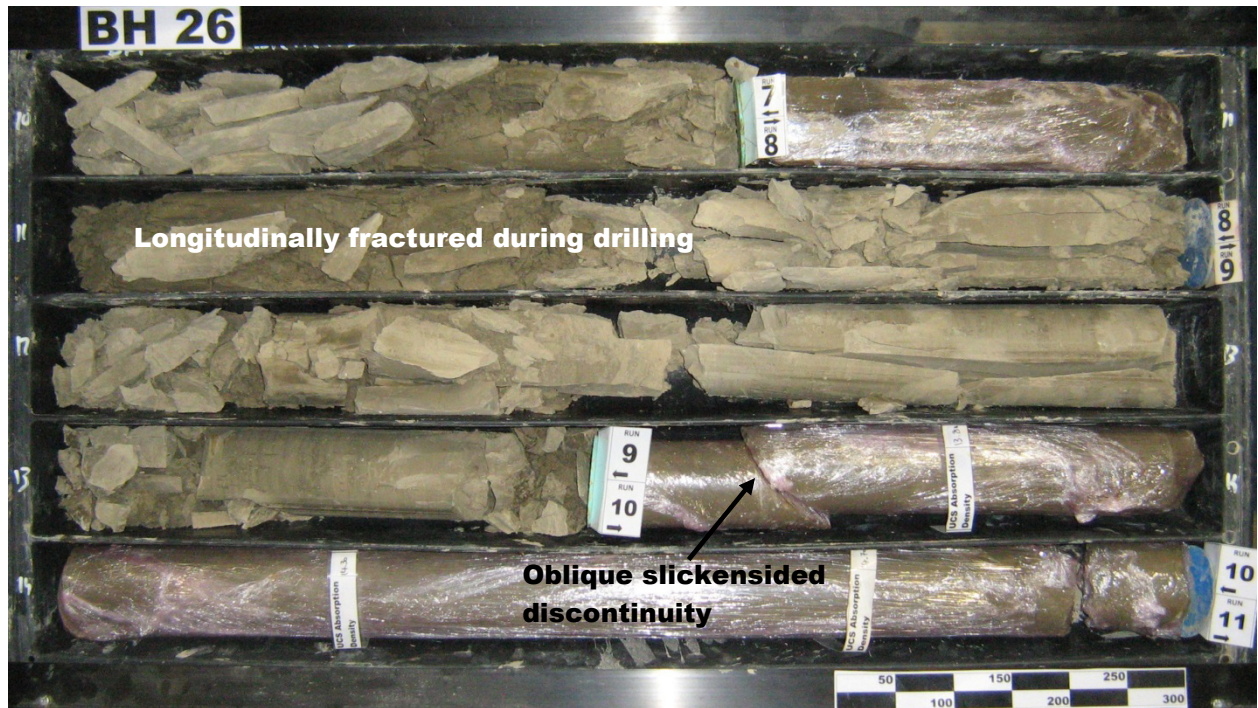
Figure 37 - example of longitudinally fractured sections of borehole core from the marl layer
