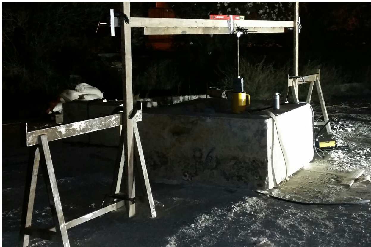
Figure 26 - Anchor pull-out test setup
